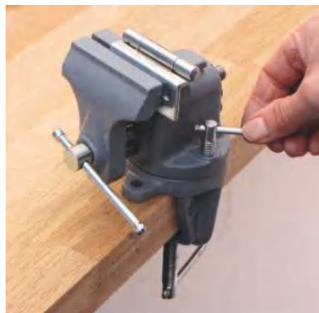
▲ A third, shorter tommy bar controls the swivel action on the vice
